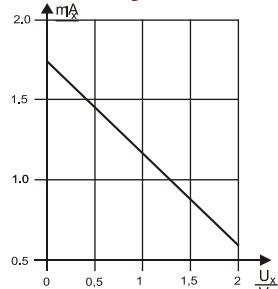
Measuring current  $I_x$  as a function of the displayed voltage  $U_x$  on the device under test.
