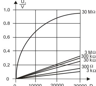
Voltage  $U_x$  across the resistance  $R_x$  to be measured as a function of measuring range and display.
